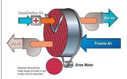
In the 1950s, Munters invented modern industrial dehumidification when it introduced the self-regenerating desiccant rotor, the heart of the dehumidifier.
