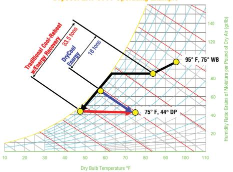
6000 cfm entering at 95°F db, 75°F wb, the DryCool ERV uses 18 tons to deliver 75°F db at 44°F dp Traditional cool-rehreat with energy recovery uses 33.5 tons to deliver the same conditions
